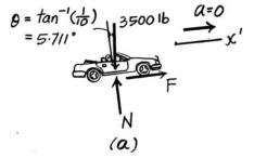
**14–59.** The 1.2-Mg mine car is being pulled by the winch M mounted on the car. If the winch generates a constant power output of 30 kW, determine the speed of the car at the instant it has traveled a distance of 30 m, starting from rest.
