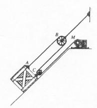
**Position - Coordinate Equation**: Datum is established at fixed pulley B. The position of point P and crate A with respect to datum are  $s_P$  and  $s_A$ , respectively.
